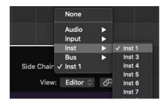
• At this point, we have a plug-in in an instrument slot, so we need a way to get sound into it. This is accomplished using the Sidechain Input pop-up in the upper-right corner - click on the appropriate category and choose the channel you'd like to process. This effectively configures Stardust as a bus effect, that is, the dry signal will be audible if the fader of the incoming track is up, so it's advisable to set the Direct Signal switch to the *Off* position.
