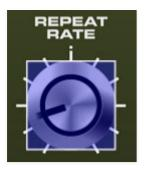
A transparent purple overlay appears over the knob, indicating that it's in learn mode. Now move the desired hardware control device. The purple overlay disappears and the hardware control will move the *Repeat Rate* knob. If you get cold feet (or accidentally put the wrong control into learn mode), learn mode can be aborted by right-clicking and selecting *Stop Learning*.
