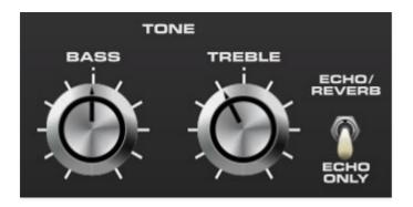
These affect the wet signals of the Tape Echo and Reverb sections. These do not affect the dry signal.
